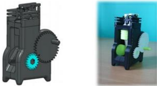
Fig 9 Images of 4 stroke engine prototype
