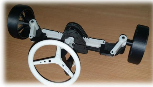
Fig 11 Images of Rack & Pinion Steering Mechanism
