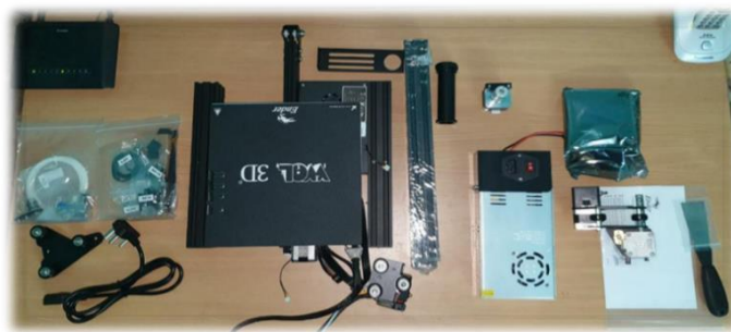
Fig. 1. Image of Disassembled 3D printer
